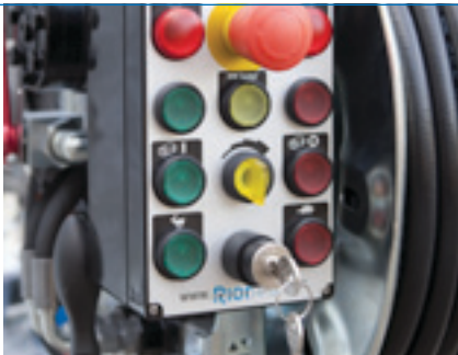
RUN-DRY PROTECTION, WITH BYPASS BUTTON
