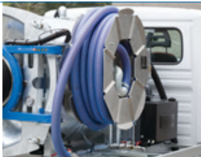
MANUAL/HYDRAULIC SUCTION HOSE REEL INCLUDING FEED BEARING
