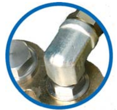
The pulsator is fastened on one of the cylinders of the pump
