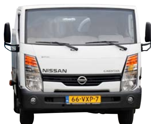
1,85 m: by lowering the cabin of the chassis and modifying the suspension
